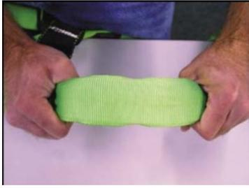
**Webbing Straps:** Grasp the webbing with your hands 6 to 8 inches apart. Bend the webbing in an inverted "U" as shown above. The resulting surface tension makes damaged fibers or cuts easier to see. Follow this procedure the entire length of the webbing, inspecting both sides of each strap. Watch for frayed edges, broken fibers, pulled stitches, cuts, burns, and chemical damage.
